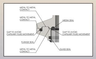
esigned to be mounted in-line for high purity hygienic applications, these clamp type "CT" sterile-design visual flow indicators provide operators with a clear view of flow for virtually any process pipeline fluid or powder. They feature an internal-flush style based on a unique O-ring seal design that minimizes traps where bacteria can buildup. Polished stainless steel sanitary clamp connections are standard with orbital weld, Swagelok TS, flange or union connections as special order items.
